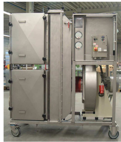
Fig. 3 left: Noble gas delay unit size S for 10 – 15 people, right: The associated airborne activity unit
