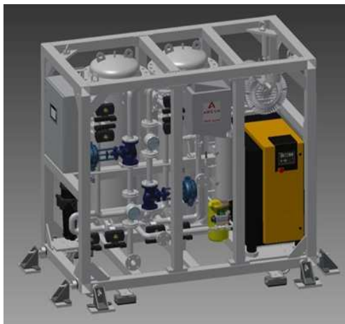
Fig. 3 left: Noble gas delay unit size S for 10 – 15 people, right: The associated airborne activity unit
